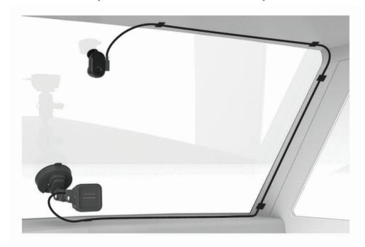
The cable is designed to be routed out of sight. To hide the cable, route it behind the vehicle trim along the windshield, doorframe, or dash.
